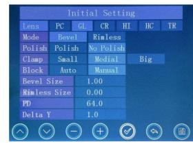
Adapt to PC,glass, Resin,HI,HC and TR lens material.
